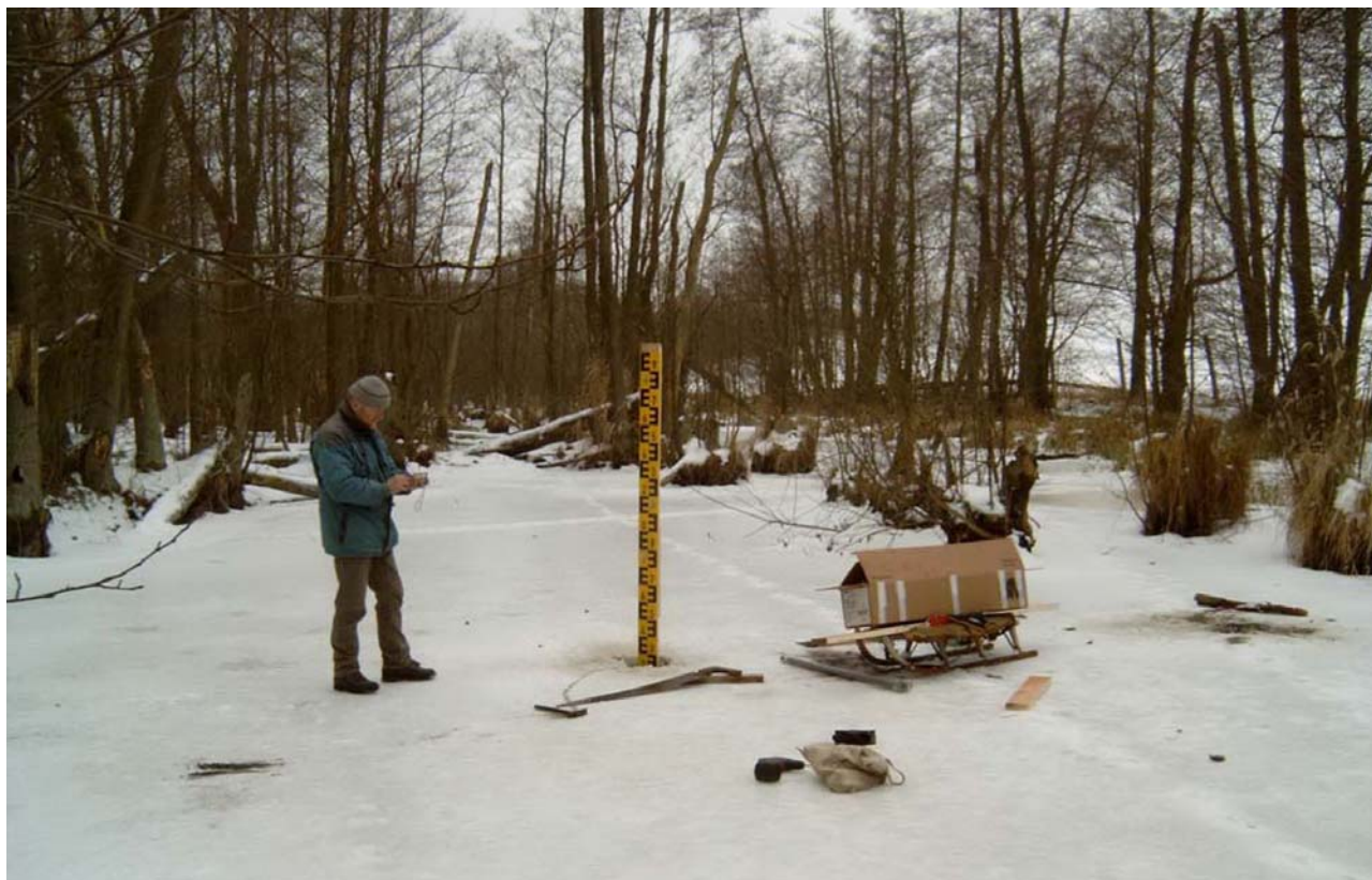
Picture 4: Setting a gauge to follow water fluctuations on turtle hibernation site
