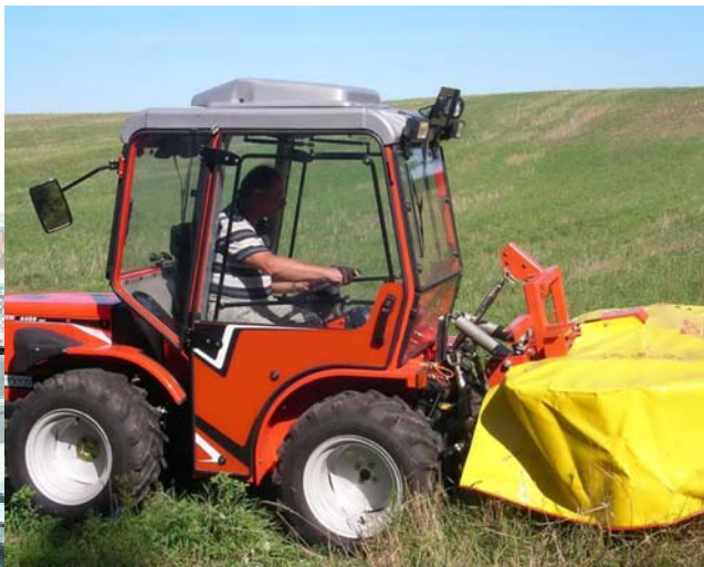
Picture 24: The vegetable-oil driven moving machine purchased to Agena on mowing mission in 2006
