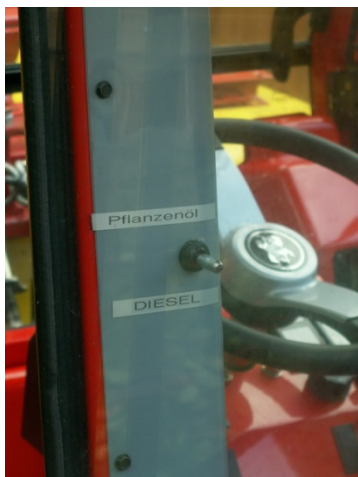
Details of the vegetable-oil / diesel switch on the mowing machine purchased to Agena
